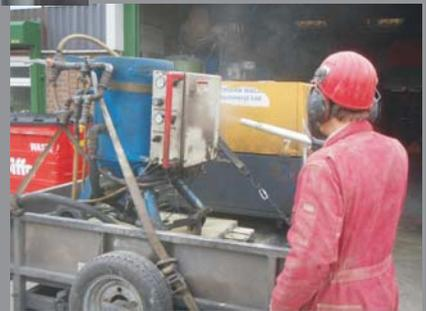
We have been providing sand blasting services for many years, but for cleanliness nothing much comes close to Dry Ice blasting as this involves no abrasive as such and a fairly minimal abrasive effect - the surface contamination is removed by thermal shock rather than abrasive scrubbing.
