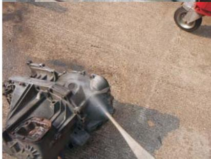
Degreasing Gearbox parts - no abrasive!
